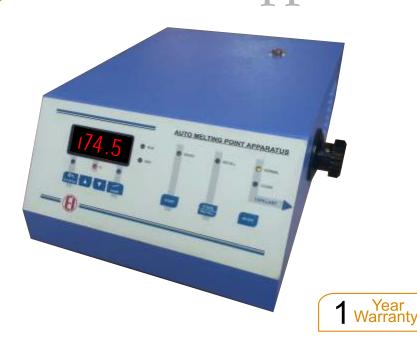
Auto Melting Point Apparatus is specially designed to find the melting point temperature of crystalline sample held within capilary tubes. Instrument uses the latest microcontroller technology and advanced engineering techniques so as to give enhanced accuracy and reproducibility.
